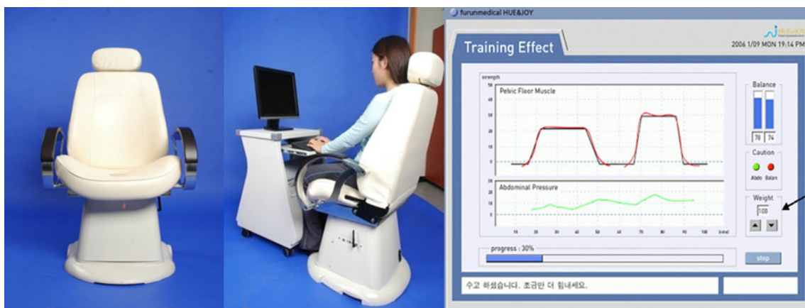
Fig. 2 Extracorporeal biofeedback device. The sensor on the center of the chair puts as much as 10 kg of pressure on the user's pelvic muscle. Responding to the physical pressure, the user recognizes the pelvic
